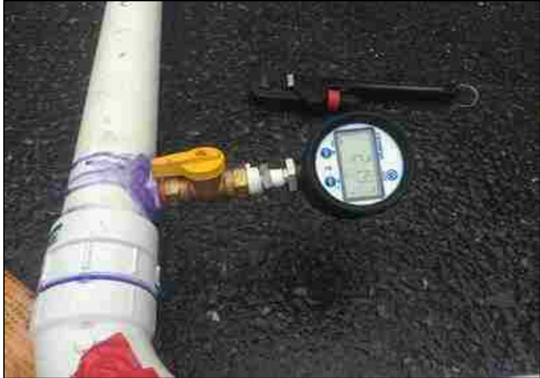
Figure 3.2: Pressure Gauge: the DPG8001 series digital measures pressure with a 0.25% full scale terminal point accuracy.
